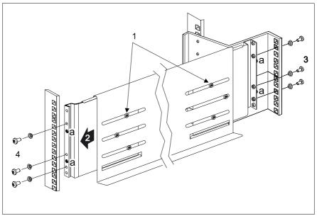
Figure 7: Mounting the left carrier rail
